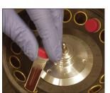
5. Centrifuge the sample for at least 120 seconds at a minimum of 12,000 RCF. Refer to your centrifuge operator's manual for centrifugation settings and times
