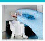
1. When the sample drawer is ready, remove the Catalyst\* whole blood separator from the sample drawer.
