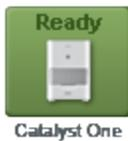
A green **Ready** icon indicates the analyzer is connected to and communicating with the IDEXX VetLab Station.
