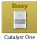
A yellow **Busy** icon indicates that the specific instrument is currently in use, either running sample tests for a different patient or running some other process, such as quality control.
